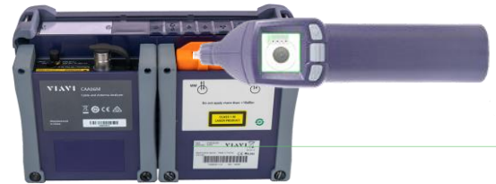
Figure 3: OTDR Port Inspection
