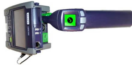
Figure 3: OTDR Port Inspection
